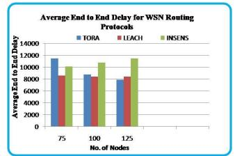
Fig. 5. Performance Comparison of Average End to End Delay for WSN Routing Protocols
