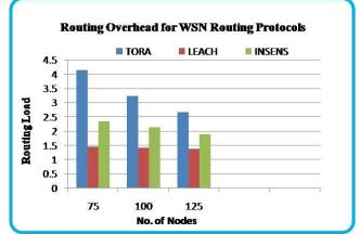
Fig. 4. Performance Comparison of Routing Overhead for WSN Routing Protocols
